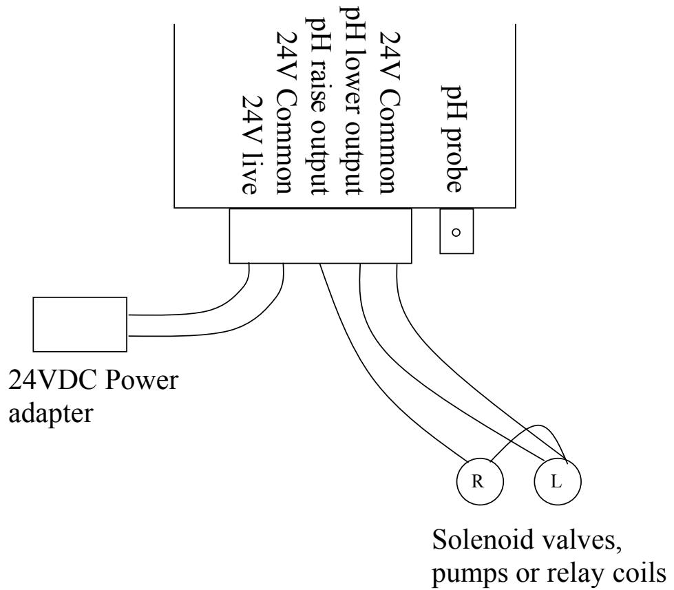
Note that all the connections marked “**24V common**” are connected together internally and you may connect the return wire from any solenoid valve or pump to any of these commons.
